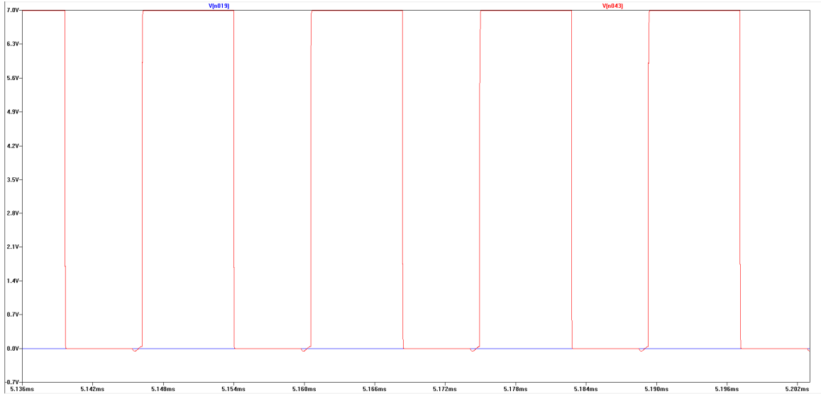
Figure 4-26: Gate Pin Voltages of LT3748 Control ICs (Discharging in Blue, Charging in Red)
