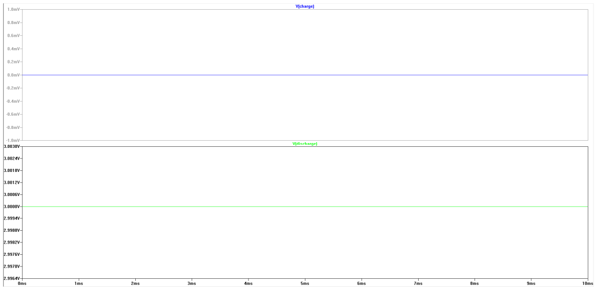
Figure 4-18: Voltage of Control Scheme when Battery Voltage is >11V and DC Bus Line >48.3V
